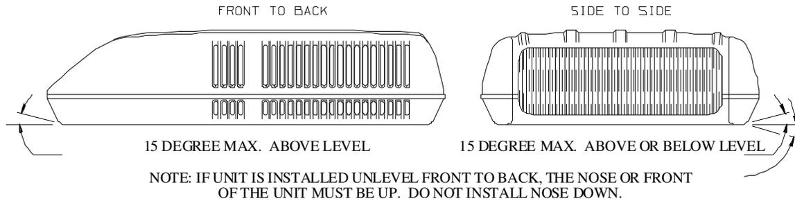
ALLOWABLE OFFSET FOR ALL HEAT PUMPS WITH ROTARY COMPRESSORS.
