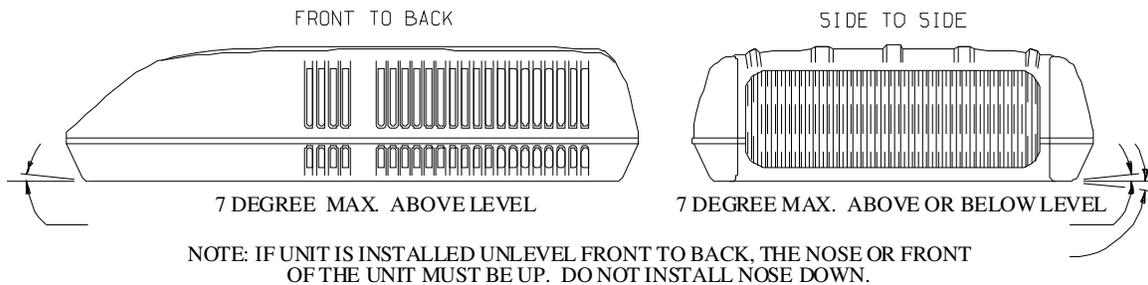
ALLOWABLE OFFSET FOR ALL HEAT PUMPS WITH RECIPROCATING COMPRESSORS.
